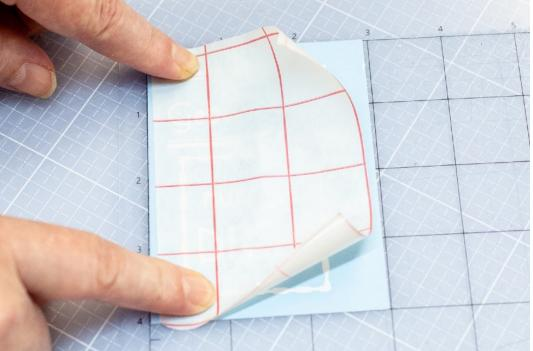
If you - as in my example - have weeded the vinyl foil while it was still on the cutting mat, you now have to remove the vinyl foil from the cutting mat. It is advisable to remove the cutting mat from the foil (and not the other way around).
