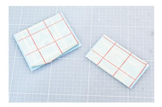
Now peel off the protective foil of the vinyl from the transfer foil. Please proceed very carefully and make sure that all parts of the motif and / or letters remain on the transfer film. Pay special attention to very small parts such as punctuation marks, i dots, etc.
